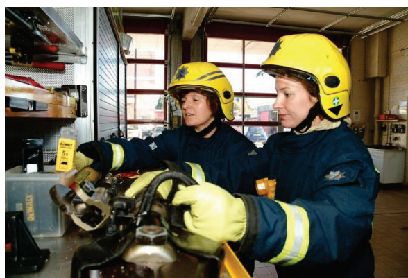
Figure 37: Routine maintenance of hydraulic rescue equipment
